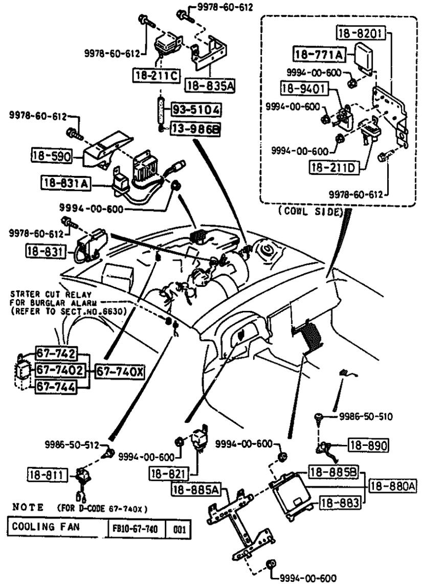
**6600BA-2 SWITCHES & RELAYS (ENGINE)
